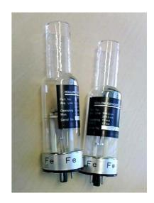
HOLLOW CATHODE LAMP WITH IRON ELEMENT
